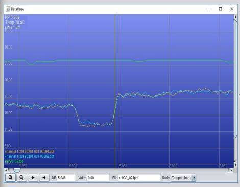
A new development presently underway is the import and display of Distributed Temperature Sensing (DTS) log data. This feature will add greater perspective when looking at hotspots or temperature anomalies in power cables as they can be easily viewed relative to the cable route, cable depth of burial and features such as subsea cable joints without having to cross reference other drawings or data. A compensation for fibre and terrain cable lengths can be applied to the Kp scale.
