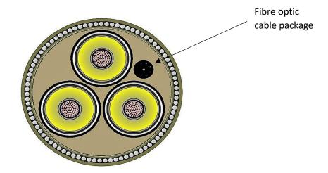
The fibre functions as a linear temperature sensor, which provides a continuous temperature profile along the entire length of the export cable.
