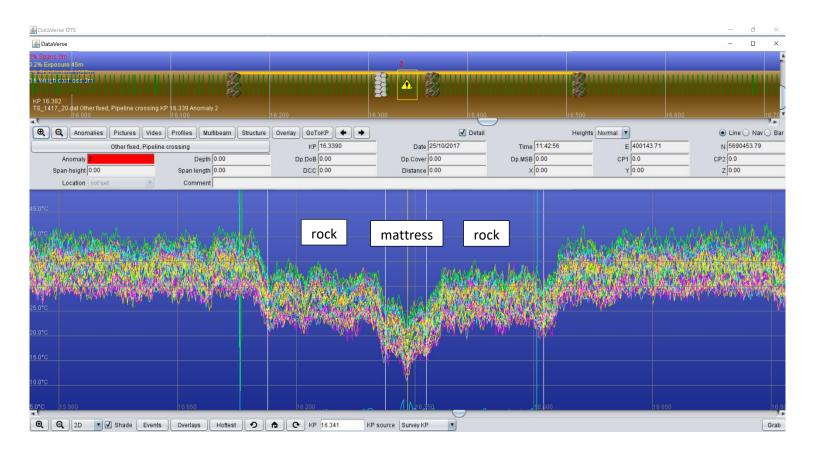
A further feature built into the Dataverse DTS viewer is the "hottest" button. The Integrity Engineer can immediately jump straight to the highest temperature recorded along the cable to save time scrolling through often huge datasets of temperature profiles. The DTS viewer can load multiple DTS files in one go and display these in a temperature graded 3D view to provide an overall perspective of the temperature trends along the route over multiple scans.
