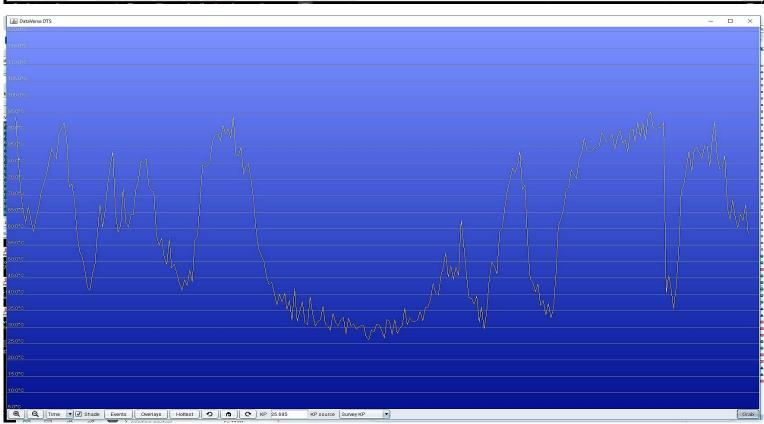
At any selected Kp you can take a time slice from the 3D viewer to show the temperature profile over time for points at that location. This provides an indication of how the temperature at a specific point on a cable changes over time. If available, current or power can be overlaid onto this to show how temperature varies with wind farm loading.
