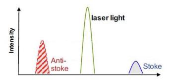
The position of the temperature reading is determined by measuring the arrival timing of the returning light pulse using Optical Time Domain Reflectometry. An Optical Time Domain Reflectometer (OTDR) operates as a one-dimensional radar allowing for a complete scan of the fibre, in this case, from only one end. The OTDR injects a short pulse of light into the fibre and analyses the backscatter and reflected signal.
